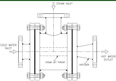
Steam Jet Heater-PI- Complete range is being offered by primetech. Steam jet heater is employed for process liquid heating application using steam as heat source. Steam jet heater employs a unique multi–port throat specially designed to admit the design steam flow rate for process heating.
