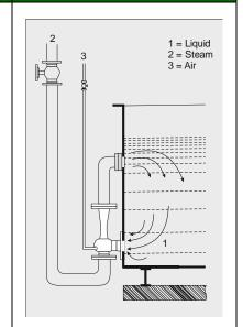
The steam jet heater is suspended in water with an inside thread connecting the steam pipe
