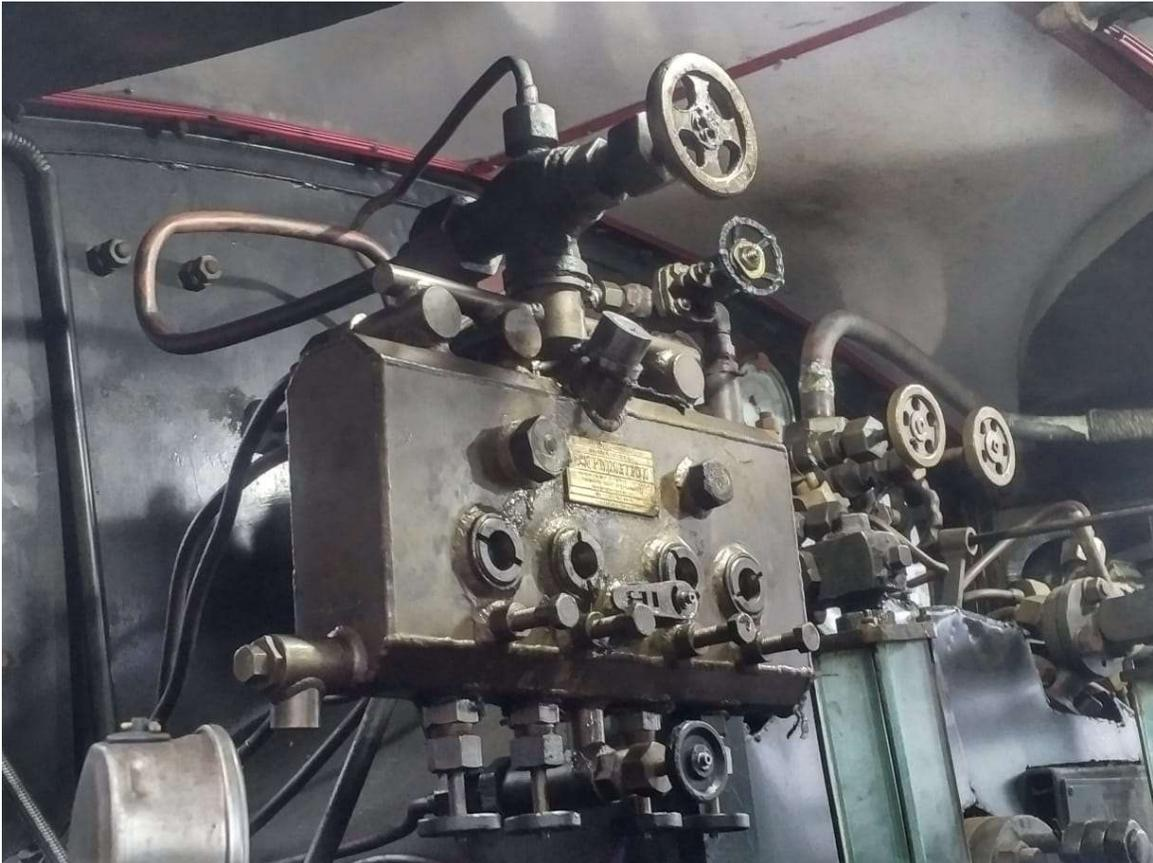
**Primetech has developed a hydrostatic sight feed lubricator in conjunction with Indian Railways to function on the heritage network. This type of four feed lubricator can be manufactured for sale world over.**
