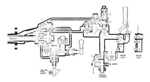
The diagram above illustrates the ejector in the" Brake Off" position, the cam (a) on the main shaft being raised to open the large ejector steam valve (b) and admit steam to the large cone (c) At the same time steam passes to the small cone (d) through the small ejector steam valve (e) This valve is set by hand so 2.s to wire draw and reduce the steam pressure to about 120 lbs., which is the pressure at which this cone is designed to give its greatest efficiency.
